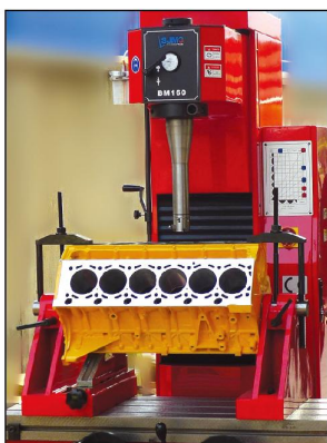
5 30° and 45° V-fixture for Boring
