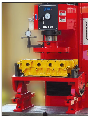
6 Universal Cylinder Head Fixture A
