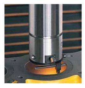
Drilling machine tool components with, respectively, a drill mounted in taper seat bush and in the drill chuck.
