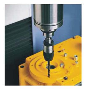
Milling an in-line block top with multiedged insert milling cutter.
