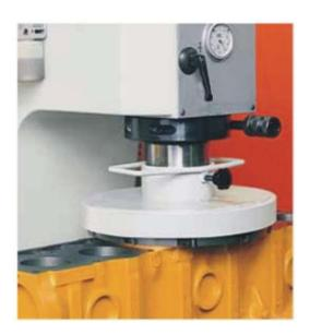
Measuring device mounted on MA 31 spindle.
