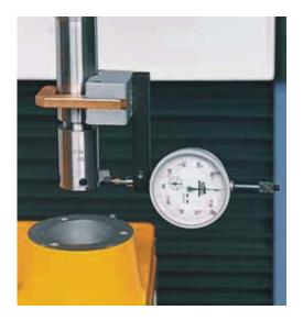
Measuring device, for setting tool out of machine.
