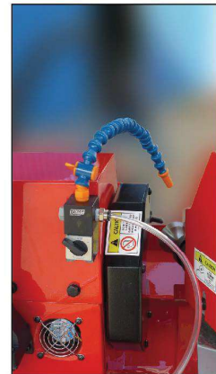
Separate Cooling System
