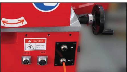
Air Pipe Port & Electric Port
