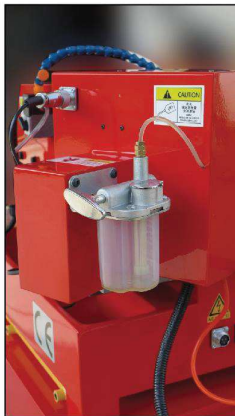
Centralization Lubrication of Fixture System
