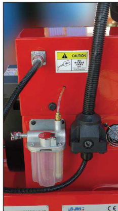
Centralization Lubrication of Grinding Wheel System
