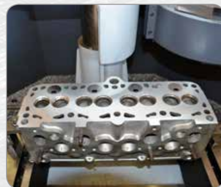
ALUMINIUM + STEEL PRE-CHAMBERS HEAD RESURFACING
